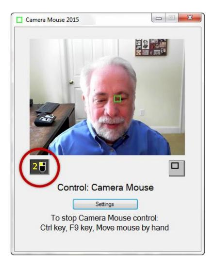
Then the user would use Camera Mouse to move the mouse pointer directly so it dwells over the Paint icon on the desktop, Camera Mouse would double-click (instead of single-clicking), and the Paint program would be opened.
