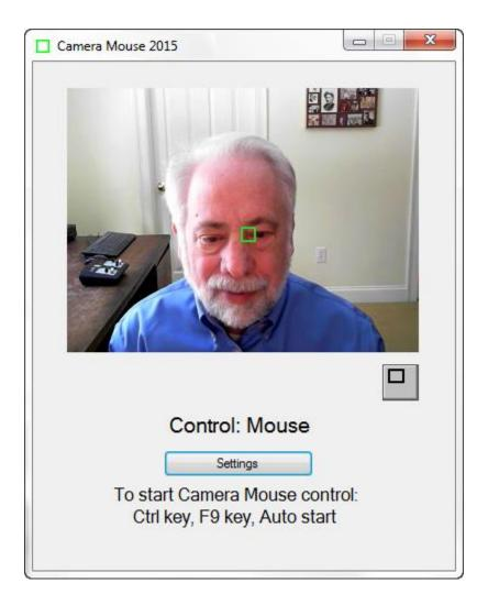
Once the feature on your face is being tracked by the computer, just press the Ctrl key or function key F9 or wait 4 seconds ("Auto start"). Now the tracking of your head should control the mouse pointer. As you move your head slowly to the right, the mouse pointer should move to the right. To return back to mouse control you can move the mouse or press the F9 key or the Ctrl key again.
