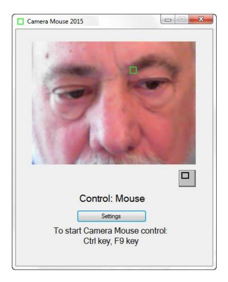
With high zoom my head fills the video image. Natural head movements cause the area being tracked to move out of the video image thereby automatically causing Camera Mouse to lose tracking, though it does reacquire usually a different track point when you move your head back in to the video image.
