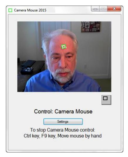
The lighting is very important. You want high contrast on the face. A bright light or bright window behind the head can darken the face and make it difficult for Camera Mouse to track. Of course the lighting can change during the course of the day and into the night. Lighting that works well at noon might not work at 5 pm or at 9 pm. You also want high contrast as the user moves or turns his head so be careful of strong lighting from one side.
