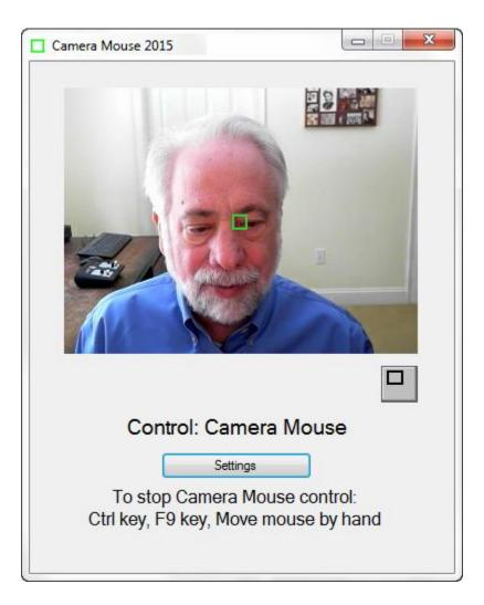
The third alternative is to have Camera Mouse automatically try to find the corner of the eye to track on start up.
